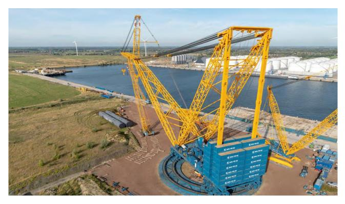
The SGC-250 is the first of the 3rd generation of ring-based cranes at Sarens. It has a maximum load moment of 250.000Tm which allows lifting an astonishing 5.000T. Even at a large radius of 100m, the crane is still capable of lifting 2.000T and, even when doing so, the ground pressure remains below 25T/m². This extremely impressive metric is achieved through the high number of wheel bogies on the double ring beams and the spreader mats that the machine features.
